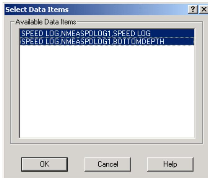
WinFrog is able to utilize the data from Doppler speed logs in the position Kalman Filter to enhance results, specifically for positioning an ROV with USBL. It is critical that the device is set-up correctly, and monitored, in order to ensure correct application of the data. It is also important to note that only the *Speed over Ground* data is used in the Kalman Filter. The Kalman Filter is under the position edit for each vehicle (the Configure Vehicle Devices dialog box).
